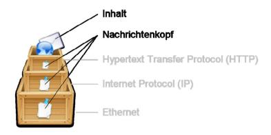
The graphic shows the nested protocol hierarchy needed to view a website on a PC, for example. Each protocol level creates a data packet out of the available information, assigns it a header (similar to an address label) and forwards the data to the next-lowest level. In this example, the ethernet packet represents the "shipping container" for transmission over the network.
